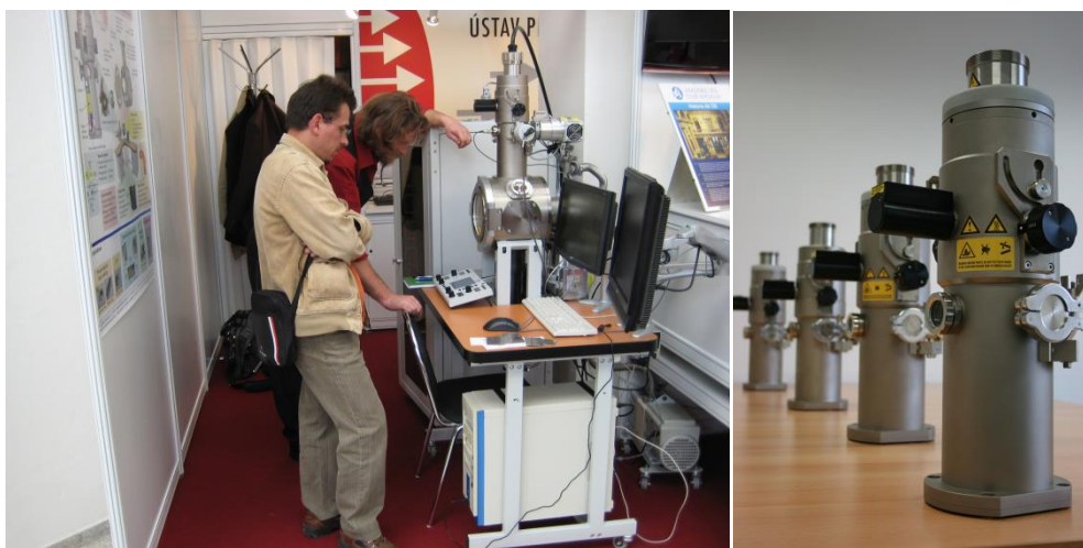
Fig. 2 The electron beam welder MEBW-60 at the International Engineering Fair in Brno in 2010 (left). The welding electron guns developed for MEBW-60 welder (right).
